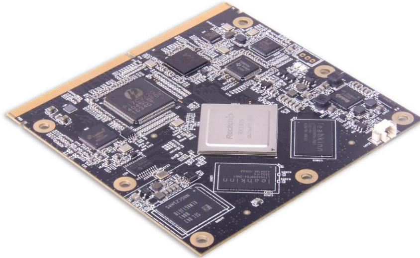
Geniatech's SoM3399-SMARC is using Rockchip 3399 processor, a high performance processor for computing, personal mobile internet devices and other applications, it integrates dual-core Cortex-A72 and quad-core Cortex-A53 with separate NEON coprocessor, is a standard module designed entirely in accordance with the SMARC2.1 specification. It is widely used in Industrial application, signages, appliances and other fields.
