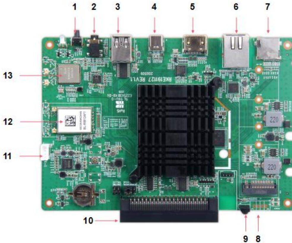
Note: Button Battery 2025 3V insert with correct polarity (+/-).
