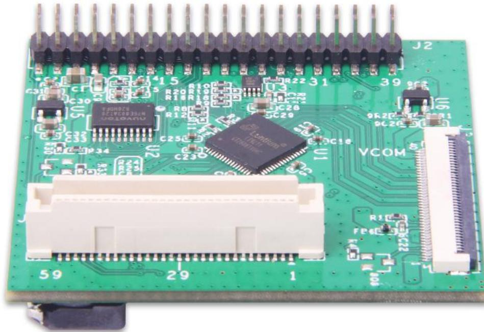
Geniatech LVDS conversion board uses LT9211 multi-channel display chip is adopted to realize various TFT display. Can realize MIPI to LVDS, MIPI to RGB, 40Pin FPC interface is provided for connecting an 8-inch TFT screen and a 6Pin FPC interface is provided for connecting a TP touch screen. LVDS conversion for DB4/DB11 enables rapid development of TFT screen applications and bulk deployment of products. Ideal for surveillance, video conferencing and even robotics projects.
