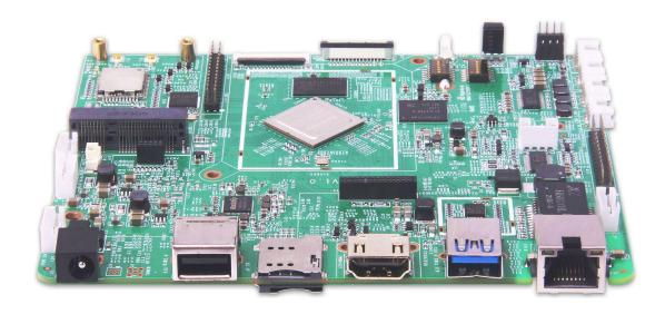
K3-3568 is a development board mainly used for commercial display equipment. With the function of tuner ,it is very convenient to watch real-time TV programs. Supporting HDMI in interface, can realize the PIP. With MIC array, it can realize AI application in the field of speech recognition. Most important ,k3-3568 has an open source SDK to help developers complete development as soon as possible.
