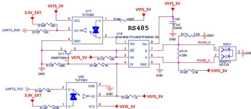
RS485 and CAN are typically selected by the jumper cap, enabling RS485 function on the 1-2 5-6 connection
