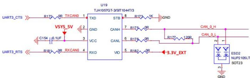
RS485 and CAN are selected by the jumper cap, enabling CAN function on the 3-4 7-8 connection
