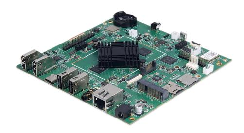
Geniatech's RK3566 Development Board Can be used for third party development or testing, can also be directly equipped with the screen, is a high cost performance motherboard
