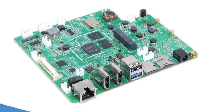
DB10 is Geniatech's latest super-performance Al 4K development board, built-in 5TOPS ultra-high computing power NPU, integrated HDMI OUT and LVDS mainstream dual display output interface, At the same time, LTE, Tuner and POE functions are added to make the functions more abundant and meet the needs of more developers in different scenarios, Commercial display, digital signage, smart home, video conference......
